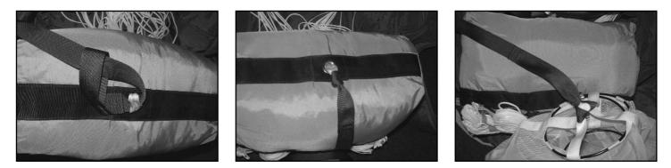
Main bag must be set into the main container, lines toward the bottom part of the container. Connecting bridle is folded up and down over the main bag. Main spring pilot chute is set over the bag and compressed by leaving netting into the spring.
