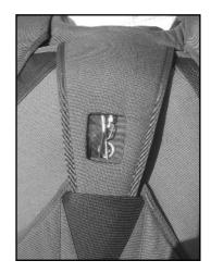
Access to breakaway and reserve ripcords, main opening system as well, are fully free and easy to be grabed. FXC control unit (if used) is free of access as well.
