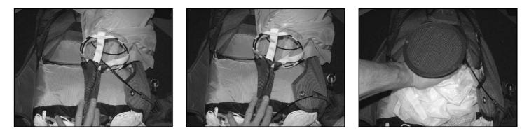
Flaps closing order is: Bottom-Up-Left and Right. To close the container insert the ripcord or static line cable into the white closing loop. Insert the remaining cable in its protecting channel if necessary.
