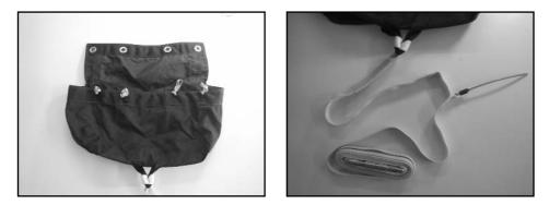
Static line must be route to the left side of the main container before closing it. The main container is secured with the cable installed on the static line.
