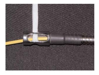
Routing of the white loop through the riser's grommet.
