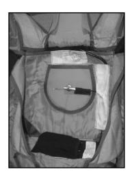
Install the A.A.D. main unit in its pocket, cable connexion must be facing downward. Airtec installation kit is only allowed for Cypres A.A.D. type. Stow remaining cables and route the cutter toward the lower reserve flap through the smallest channel. Control unit must be route in the white type 4 / 1.5" channel toward the collar.
