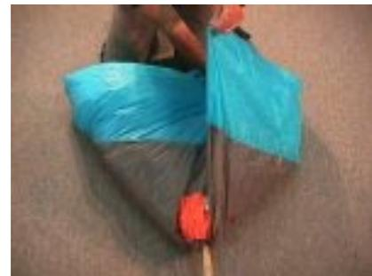
Fold the “ears” in so that the entire canopy is bag width. Pull the bridle attachment out to one side or the other.
