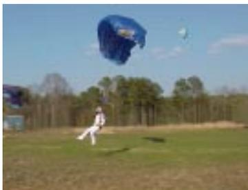
All Icarus canopies, have constant cell proportion (CONSTANT CELL ASPECT RATIO): As the canopy chord narrows toward the tips, so does the height and width of those cells. Making the cells proportional makes and maintains the airfoil shape better than the old construction techniques. This creates better balance and symmetry in the canopy, which results in better openings, better control, better performance and nicer overall manners.
