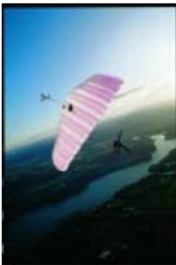
These canopies seem generally conventional in design in that they are made from nine two-chambered cells. What separates Icarus Canopies from previous designs is a construction technique that makes them more like a true aircraft wing than a parachute.
