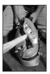
Finish the lines stowage by keeping tension on them. Length of lines after the band must not exceed 5 cm. Check that lines are not crossing each other.
