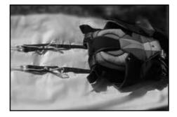
At this point, go toward the canopy and free it from main pilote chute, bag and briddle. Look at the trailing edge and go to the steering lines. Take each of them between your fingers and untwist them by rolling the line between your fingers down to the toggles.
