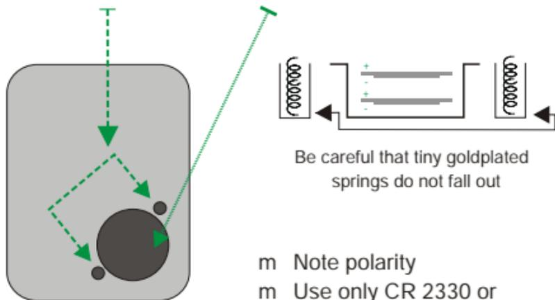
Note: After removal wait 120 sec. before installing new batteries.
