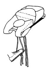
After the pull-ups have been pulled all the way through the bottom of the container, their ends can be tied together. Then with the rig placed at the edge of the packing table, it will be possible to step into the resulting loop with one foot, creating enough force to close the container with little effort.
