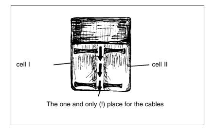
Finally, replace the top of the compartment in its original position, so that the two screws protruding downward fit securely into their holes in the bottom of the compartment, without forcing. Tighten both screws with approx. four cautious clockwise turns, once their threads have been engaged.
