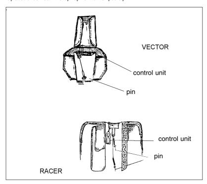
The control unit should be attached using the four small nylon ties built into its bottom surface. These ties can be pulled through nylon layers with a needle and then secured with appropriate knots.
