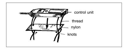
Alternatively the transparent pouch (supplied with the installation kit) can be hand sewn or machine stitched under the reserve top flap. The control unit is then pushed into the pouch and not sewn directly to the rig.
