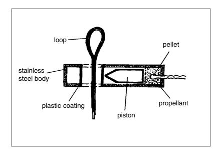
The distance which the piston moves in case of an activation is approx. 5 mm.
