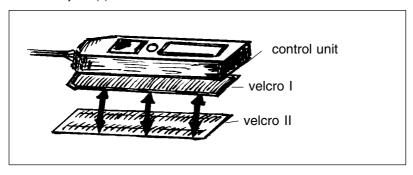
Once the control unit has been mounted, make sure that it cannot interfere with the reserve container opening, the ripcord, the pin(s).
