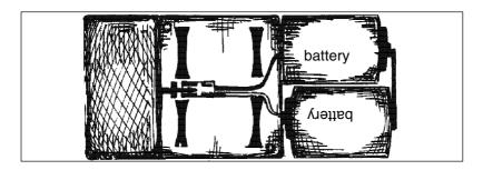
Then, position both battery cells between your thumb and index finger on their right and left sides, and turn them upside down toward the unit's closed casing until they are in a position exactly overhead the opened battery compartment. From this horizontal position, they can now be lowered straight into the battery container.
